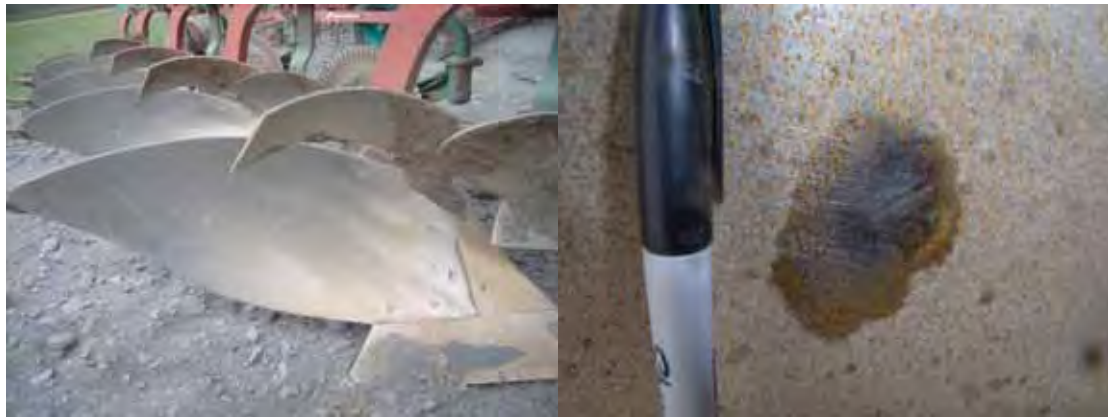
Figure 4: Corrosion of new ploughing machinery at Porvaldseyri farm, approximately 8km southeast of the volcano. This corrosion took place overnight.
